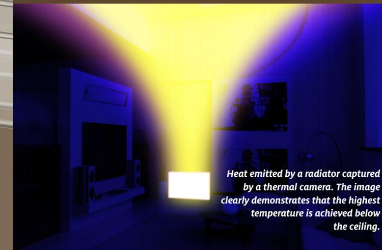
Heat emitted by a radiator captured by a thermal camera. The image clearly demonstrates that the highest temperature is achieved below the ceiling.
